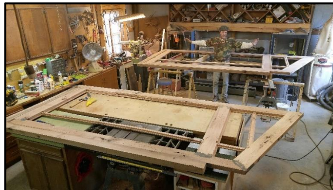
Woodworking Shop with Rusty Rothgeb working on The MobbyMac Oak Doors that were milled, dried, and fabricated at Rockspire. This shop is where all the sawing, drilling, carving, turning, grinding, and chipping projects are completed. Anything that creates saw dust or chips, happens here.
